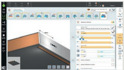
When the parameter is selected, the dimensions are displayed on the workpiece.
