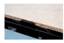
The protection boards or pallets are aligned fully automatically during infeed into the system to ensure optimum stack formation
