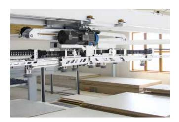
The ST71 suction cross rail in X geometry is the ideal optional feature for panel storage. The self-learning cross rail generates the data required for panel handling independently and thus ensures dependable process reliability. The operator does not have to enter anything.
