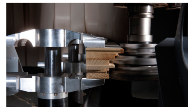
Liquid-cooled trimming spindles with vector control
