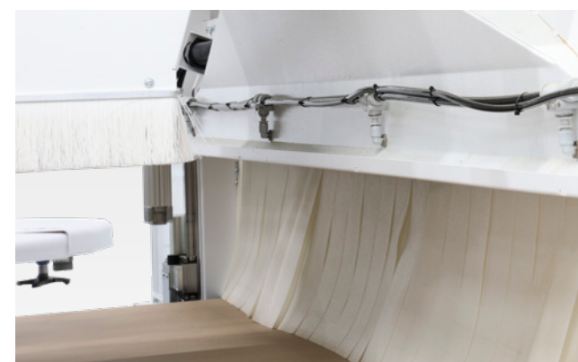
Combined suction and pushing device
