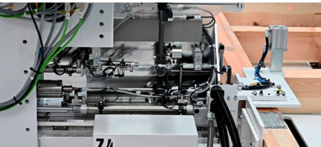
Screw unit for screwing frame works together.
