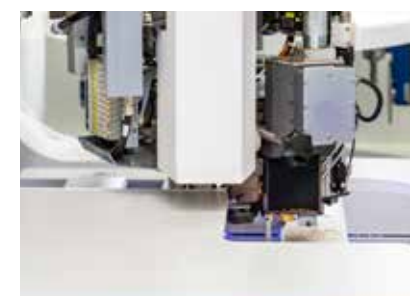
oklejanie 360° agregatem powerEdge Pro Duo
