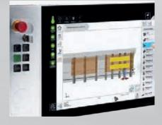
Second operating terminal (option) for optimum shuttle operation without unnecessary walking – ideal for machines with a large work field. Program selection and assignment of the machine is possible on both sides.
