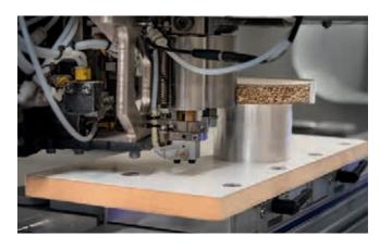
$360^{\circ}$  edge gluing with the powerEdge Pro Duo edge banding unit
