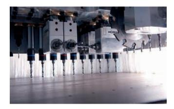
High-speed drilling technology with groove saw
