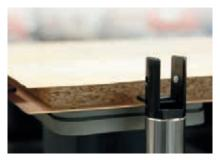
Stop pin for covering layer overhang with end position monitoring to protect tools, units and machine operating personnel.
