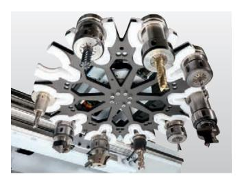
10-space tool changer traveling with spindle. Tool change during drilling or edge banding. For tools and units with a diameter of up to 180 mm.
