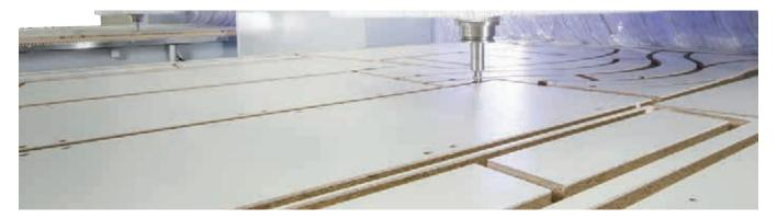
Nesting processing of panel materials: waste-optimized cutting to size and processing in the surface
