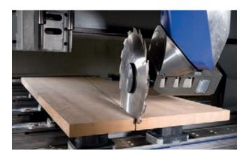
Separating cuts up to 110 mm in height
