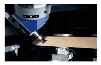
Routing a burr connection for jamb/rail designs
