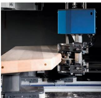
**Pneumatic interface** – the patented interface with 3-way support on all C-axes and 5-axis heads enables the use of traced units, e.g. for precise rounding off at the top and bottom no matter the thickness tolerances.
