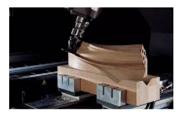
Routing a staircase handrail
