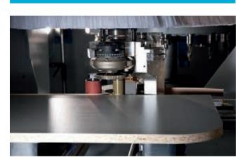
easyEdge gluing unit for rational gluing on shaped parts
