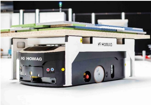
Image 10: At 1240 x 695 mm, the TRANSBOT is a compact, high-performance solution. It transports a maximum weight of 1200 kg at a travel speed of up to 60 meters per minute.
