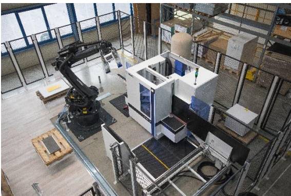
Image 1: DRILLTEQ V-500 and FEEDBOT D-300 combine to form an efficient production cell.
