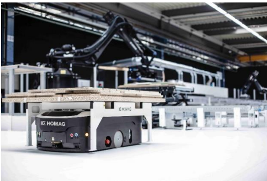
Image 11: Each TRANSBOT also detects people and objects in its travel path using the in-built laser scanner for navigation, thereby ensuring safety during operation.
