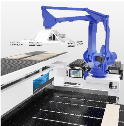
Image 7: SAWTEQ B-300 flexTec. The saw can be operated manually, but a fully automated batch size 1 cutting process is also possible thanks to the integrated robot.
