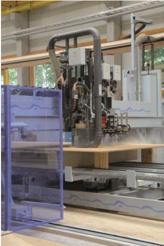
Picture 8: Multifunctional bridge WMS 120 while processing the sheathing like cut-outs for windows.
