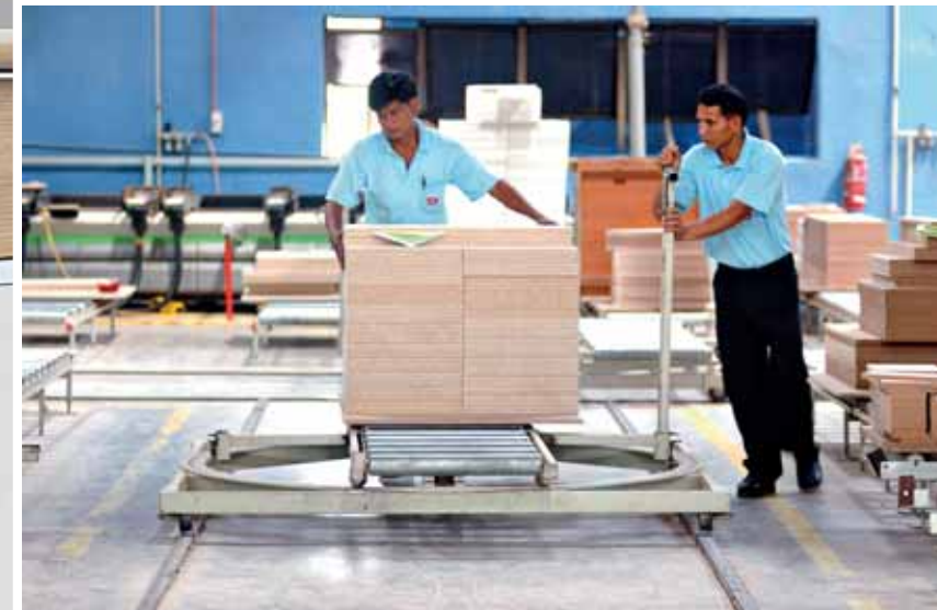
On the way to the customized production Versalink and Schuler defined together different development steps. Seen in the picture is the transport via Roller Conveyor.
