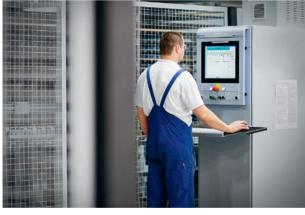
3 — Controlling the buffer Employees can monitor the parts leaving the storage area and the sorting buffer in real time on a screen.
