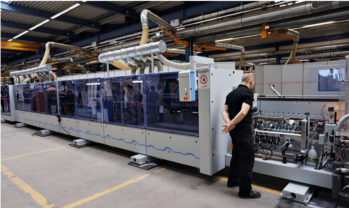
Fig. 3: Rear part of the rebate edge machine from the softforming units
