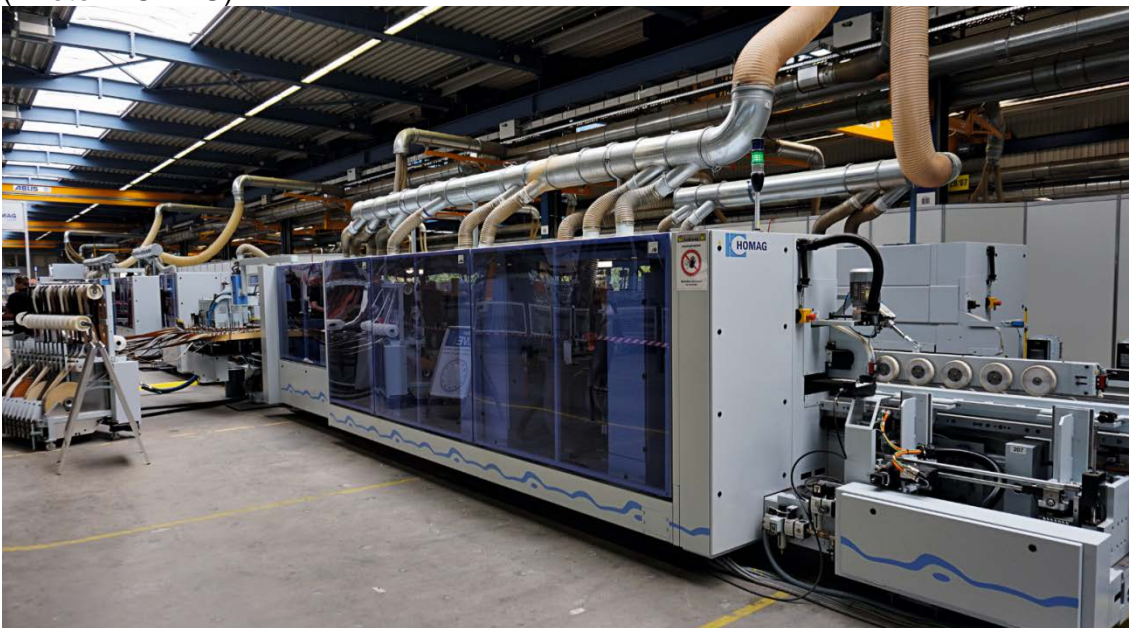
Fig. 2: The front part of the rebate edge plant with the reference edge trimming unit and the KFL623 rebate edge machine at the front up to the edge magazine
