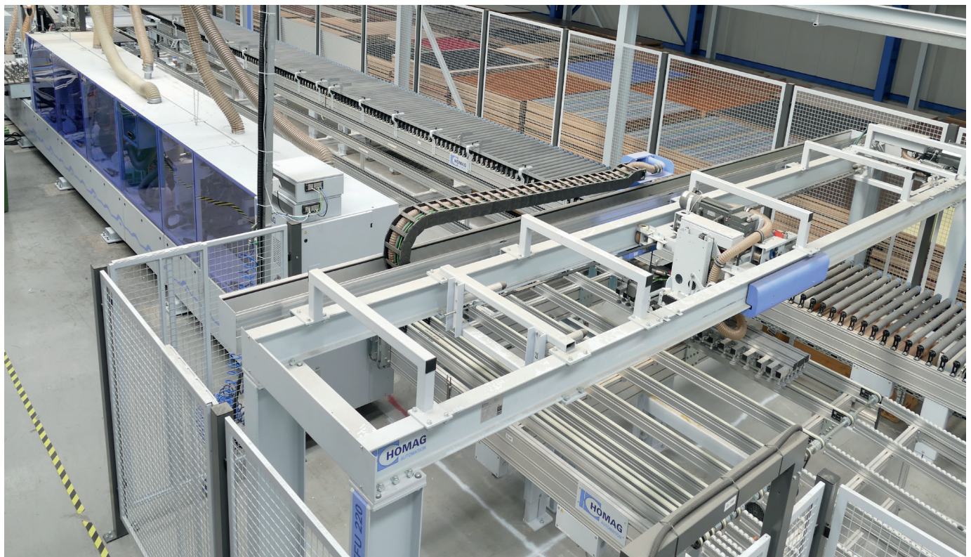
Edging cell in the foreground, storage system behind
